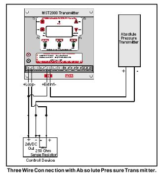
The MST2000 with Ab so lute Pres sure Trans mit ter can be wired to re place your existing three wire trans mitter.
